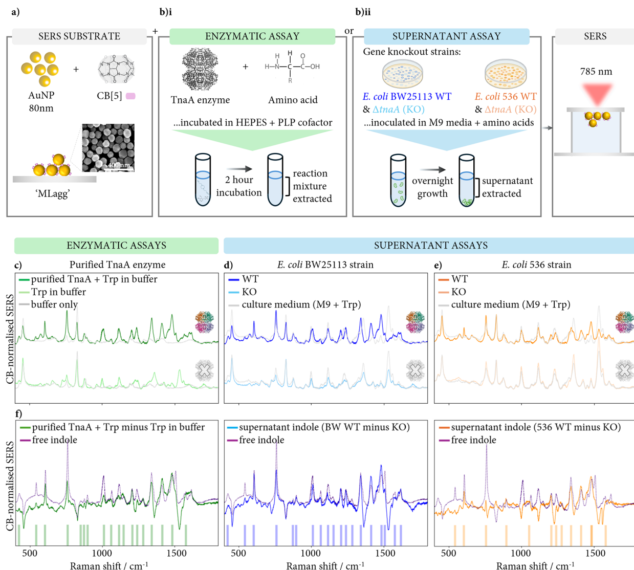
Figure 1. In vitro and in vivo SERS characterization of TnaA-dependent indole production in E. coli . (a) SERS sensing films, from aggregation of 80nm gold nanoparticles with CB[5] molecules at a liquid–liquid interface before drying into films. 45 (b) (i) Enzymatic assays which incubate the purified enzyme TnaA and amino acid in HEPES buffer and PLP cofactor; (ii) E. coli grown overnight in media containing M9 media supplemented with amino acid (see Methods). Supernatant is extracted and SERS measured. (c–e) Normalized SERS spectra of (c) enzymatic assay of TnaA combined with tryptophan (dark green), an identical solution without the enzyme TnaA (light green), and buffer solution only (without tryptophan, gray); (d) E. coli BW25113 and (e) E. coli 536 of both wild-type (WT) and tnaA gene knockout strains (KO, \Delta tnaA ), together with culture media of M9 media supplemented with tryptophan shown for reference (gray). (f) Subtraction of the two spectra shown in (c–e) and comparison to the spectrum of 10mM free indole. Significant peaks shown as shaded vertical lines, demonstrating strong alignment between the spectra and the presence of supernatant indole in these assays, as confirmed by mass spectrometry (see Figure 4).
