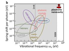
$|\gamma_{\nu} - \Gamma_{tot}(l_l)| = \gamma_{\nu}/2$  over the detuning range. Box shows the results for the NPoM including the full multimode plasmonic response, as considered in the simulations, and with  $\omega_c$  fixed at the NPoM dark-field resonance of 800 nm, giving -10-fold enhancement. **b** Comparison of spring shifts per cavity photon *vs*  $\omega_v$  for a range of systems<sup>50</sup>.
