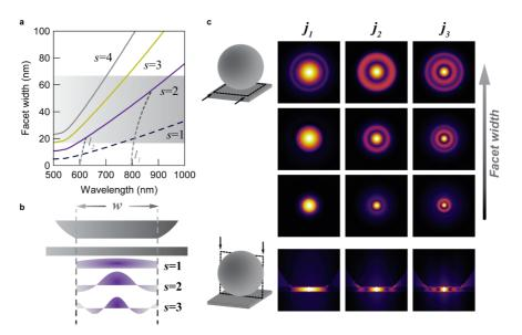
Figure 2. MIM waveguide model. (a) Dispersion of MIM waveguide with s = 1,2,3,4 modes for varying facet size. Shaded area shows experimentally accessed facet range. (b) 1D MIM waveguide with boundary conditions defined by the facet size. (c) Lateral normalized field distribution  $|E|^2$  for first three modes seen in the nanogap of Figure 1d for increasing facet widths from 10 to 30 nm (top 3 rows) and vertical field distribution of 30 nm facet (bottom).
