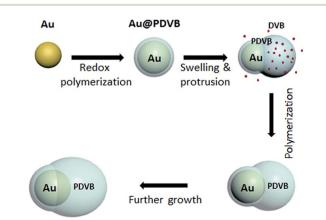
Scheme 1 Formation of anisotropic hybrid nanoparticles made of Au–PDVB. The yellow sphere is the AuNP and the red dots represent DVB monomers, which swell, crosslink and enlarge the light blue region representing the PDVB coating.
