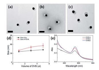
Fig. 3 Size of hybrid Au-PDVB hetero-dimers with increasing DVB of (a) 1  $\mu$ l, (b) 3  $\mu$ l, and (c) 5  $\mu$ l, while keeping 0.6 mM concentration of HAuCl<sub>4</sub> fixed. Scale bars are 100 nm. (d) Size dependence of Au and DVB components of hybrid nanoparticles vs. DVB volume, with (e) corresponding absorption spectra.
