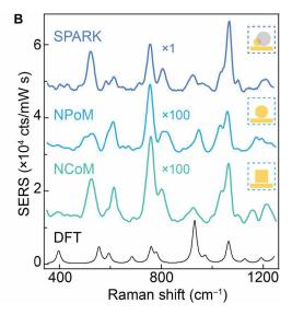
Fig. 1. Plasmonic cavity for MPA SERS sensing. (A) Self-assembled MPA monolayer (blue) sandwiched in NPoM (top) and SPARK (bottom) geometries. Red arrows indicate optical in- and out-coupling angles. (B) Time-averaged SERS spectra of the MPA monolayer collected from SPARK, NPoM, and NCoM nanocavities with, respectively, 20-μW, 500-μW, and 1.2-mW optical excitation at 633 nm (300 s integration time), together with simulated Raman spectrum for monodentate MPA using polarized DFT calculations.
