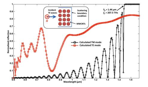
207.5 THz with corresponding plasma wavelength of  $\lambda_p$  = 1.44  $\mu$ m were calculated using Eq. (1). The value of the frequency dependent permittivity for the structure was calculated from Eq. (2). From Ref. 2, the reflection coefficient at normal incidence for such metamaterial can be calculated using Fresnel equations as
