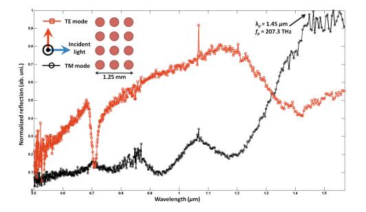
FIG. 3. (Color online) The reflection measurement from the sample for light polarized parallel (TM) and perpendicular (TE) to the MWCNTs. A sharp drop in the reflected TE-mode is observed at plasma frequency ( $\lambda_p$ =1.45  $\mu$ m) which matches well the theoretical result. No such cutoff effect is observed for the TE-mode.
