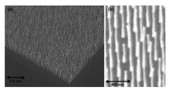
FIG. 2. (a) Electron microscopy image of a 2D square lattice array of MWCNTs having radius of 50 nm and lattice constant of 400 nm, grown on silicon substrate using PECVD. (b) The same in higher resolution.
