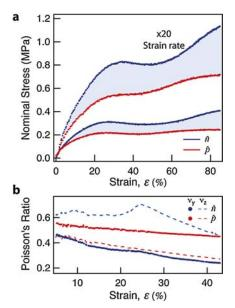
FIG. 2 (color online). (a) Stress-strain curves for strips stretched along the  $\hat{p}$  and  $\hat{n}$  directions, at rates of 10 and 200  $\mu$ m s<sup>-1</sup>. (b) Poisson's ratio in-plane (y) and perpendicular to the plane (z).
