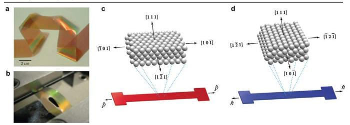
FIG. 1 (color online). (a) Unmounted opal roll and (b) mounted opal strip in strain rig, showing structural colors. (c),(d) Strip oriented in  $\hat{p}$  directions is stretched (b) along or (c) perpendicular to lines of spheres.
