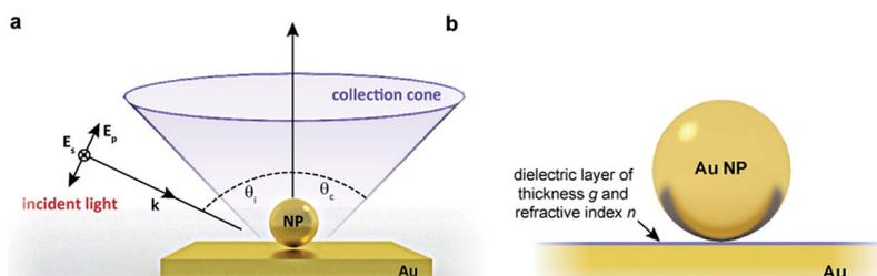
Fig. 4 The FDTD simulation geometry. (a) Particle illuminated with s- and p-polarized plane waves at angle  $\theta_i$  and scattered light collected over a cone with half-angle  $\theta_c$ . This replicates the experimental dark-field geometry. (b) Molecular or semiconductor monolayer in the gap modelled as an infinite dielectric sheet of thickness  $g$  (which determines the gap) and real refractive index  $n$ .
