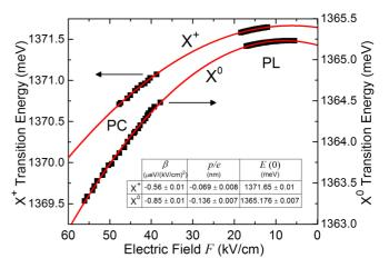
FIG. 2. Plot of the  $X^0$  and  $X^+$  transition energies as a function of F obtained through both PC and  $\mu$ -PL spectroscopy. Equation (1) is fit to the experimental data (solid lines), yielding precise values for p,  $\beta$ , and E(0), which are given in the table in the inset.
