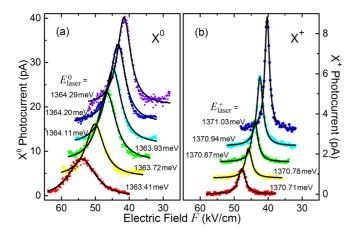
FIG. 1. Single-QD PC spectra of (a)  $X^0$  and (b)  $X^+$  for a series of values of (a)  $E^0_{\rm laser}$  and (b)  $E^+_{\rm laser}$  with Lorentzian fit curves (solid lines). For clarity, spectra are shifted vertically with respect to each other.
