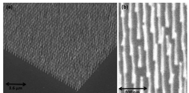
FIG. 2. (a) Electron microscopy image of a 2D square lattice array of MWCNTs having radius of 50 nm and lattice constant of 400 nm, grown on silicon substrate using PECVD. (b) The same in higher resolution.
