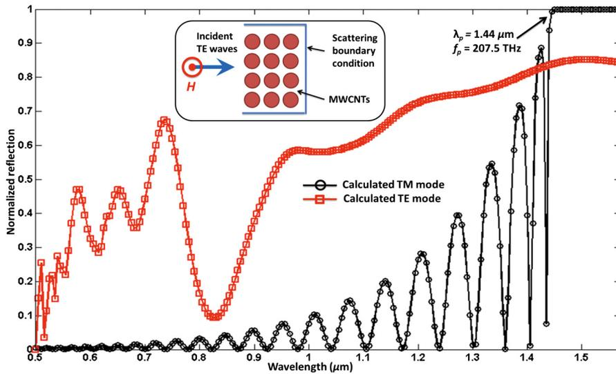
FIG. 1. (Color online) The calculated TM and TE reflection spectra for MWCNT based high pass filter. In TM-mode the incident light is polarized parallel to the wire structures and at the plasma frequency  $f_p$  of 207.5 THz ( $\lambda_p=1.44 \mu\text{m}$ ) a sharp drop in reflectivity is calculated. The inset shows the boundary conditions of the FEM model simulated to calculate the TE reflection spectrum.
