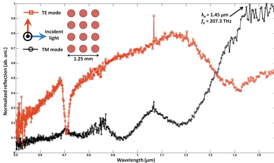
FIG. 3. (Color online) The reflection measurement from the sample for light polarized parallel (TM) and perpendicular (TE) to the MWCNTs. A sharp drop in the reflected TE-mode is observed at plasma frequency ( $\lambda_p = 1.45 \mu\text{m}$ ) which matches well the theoretical result. No such cutoff effect is observed for the TE-mode.
