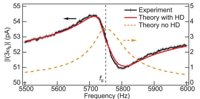
FIG. 2. (Color online) Measured  $|I(3\omega_s)|$  (solid markers) vs. numerical simulation with the same parameters and HD included (solid line) and absent (dashed line). The frequency used for alignment scans is  $f_s$ .
