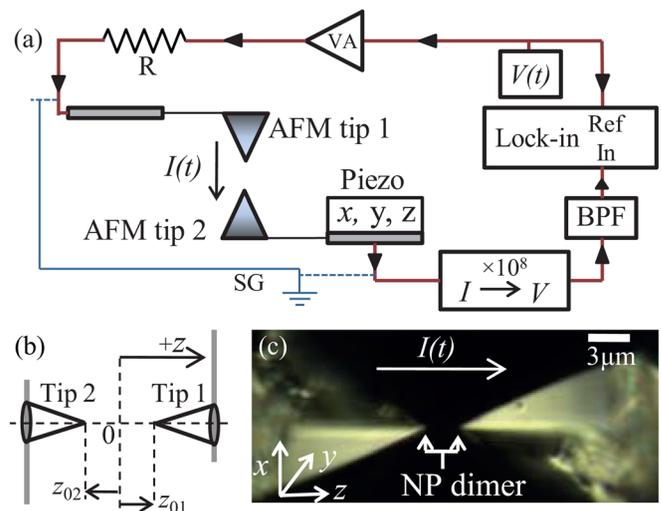
FIG. 1. (Color online) (a) Experimental setup with signal ground (SG), BPF, and voltage amplifier (VA). (b) Coordinate system used in theoretical analysis. (c) Dark-field image of metal coated AFM tips.
