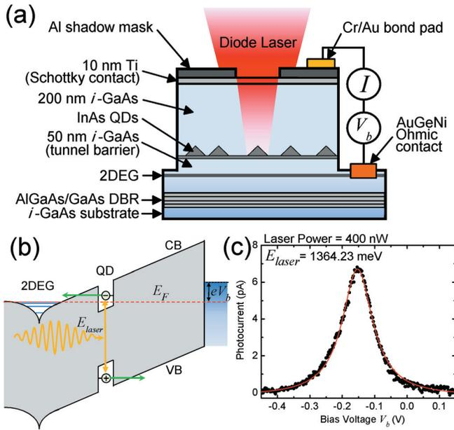
FIG. 1. (Color online) (a) Schematic diagram of the  $n$ - $i$ -Schottky photodiode used for single-QD PC measurements. (b) Energy-level diagram using resonant laser-excitation. (c) Single-QD  $X^0$  PC peak obtained by sweeping the  $X^0$  transition energy through a fixed  $E_{laser}$  via the QCSE. For this PC peak,  $E_{laser} = 1364.23$  meV and the laser excitation-intensity is 400 nW. The solid line is a Lorentzian fit.
