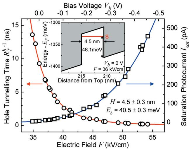
FIG. 3. (Color online) Plot of  $I_{sat}$  (squares) and hole tunnelling time  $R_T^{-1}$  (circles) as a function of  $F$ . The solid lines are fits using the theoretical model based on a 1D WKB approximation in Eq. (2), yielding  $H = 4.5 \pm 0.3$  nm and  $E_b = 40.5 \pm 0.3$  meV. Inset: Theoretical calculation of the valence band and QD  $s$ -shell hole eigenvalue using a 1D self-consistent Poisson-Schrödinger solver.
