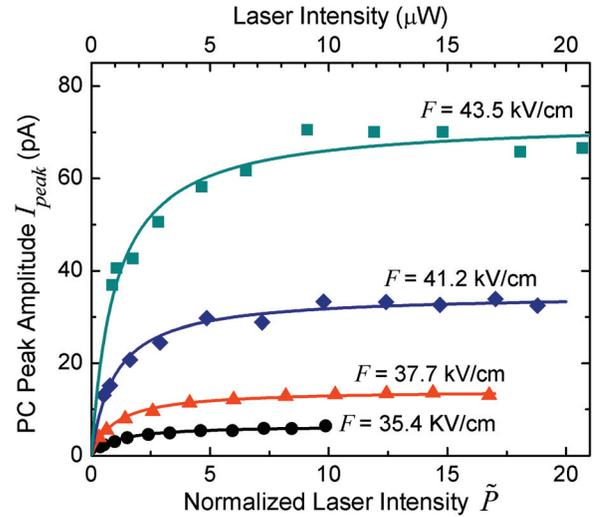
FIG. 2. (Color online) Plot of the PC peak amplitude  $I_{peak}$  as a function of normalized laser excitation-intensity  $\tilde{P}$  for  $X^0$  resonance peaks centered at several values of  $F$ . The solid lines are fits using the theoretical model of Eq. (1).
