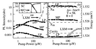
FIG. 2. (a) Normalized perpendicular PL emission vs  $I_{\text{pump}}$ , for polariton modes ( $\bullet$ ) and the localized-exciton lasing mode ( $\bigcirc$ ). Inset: expected normalized PL for spatially inhomogeneous Rabi transition; (b) peak perpendicular PL emission energies vs  $I_{\text{pump}}$  for polariton modes ( $\bullet$ ) and the localized-exciton lasing mode ( $\bigcirc$ ). The detuning,  $\Delta$ =-3 meV.
