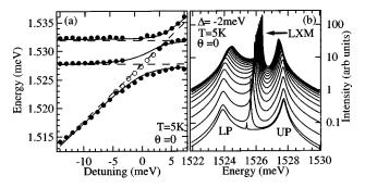
FIG. 3. (a) Experimental PL emission of upper, middle, and lower polariton modes ( $\bullet$ ) and the localized-exciton lasing mode ( $\bigcirc$ ) together with theoretical dispersions of upper, middle, and lower polariton modes (solid lines), cavity,  $X_{hh}$  and  $X_{lh}$  modes (dashed lines), shown vs cavity detuning; (b) calculated emission from weakly and strongly coupled states. The pump evolves from 200  $\mu$ W to 3 mW in steps of 200  $\mu$ W.
