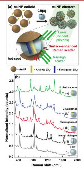
**Figure 2.** (a) Schematic of host–guest SERS analysis using ternary complexation: CB[8] aggregates AuNPs and localizes the analyte (G<sub>2</sub>) in the hot-spot for SERS analysis. (Note: The AuNPs are not drawn to scale with the analytes.) (b) SERS spectra of (i) CB[8] (5  $\mu$ M); (ii)–(v) CB[8] complexes. SERS signals from both CB[8] and guest molecules are observed in the CB[8] complex spectra. (Note: spectra are stacked for clarity.)
