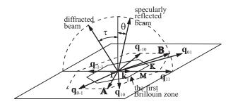
Fig. 2. The first Brillouin zone and the photons wavevectors. Plane of incidence is along  $\Gamma - M$  direction.
