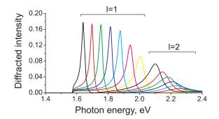
Fig. 5. Calculated intensity of the first-order diffracted beam with in-plane wavevector  $\mathbf{q}_{-1,-1}$  versus photon energy  $\hbar\omega$  for a surface of nanoporous gold formed by a hexagonal arrangement of spherical voids of different diameter *d*: from 380 to 500 nm (from right to left, in steps of 20 nm). The angle of incidence is 50°. The lattice constant ( $|\mathbf{a}| = 515$  nm) is kept unchanged in these calculations.
