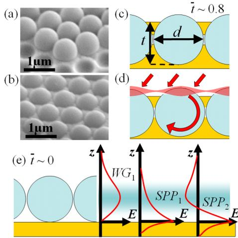
FIG. 1 (color online). (a), (b) Angled electron micrographs of  $d = 700$  nm spheres at (a)  $\bar{t} = 0.15$ , (b)  $\bar{t} = 0.55$ . (c) Schematic film cross-section for normalized thickness  $\bar{t} = t/d$  for thickness,  $t$ , and diameter,  $d$  of  $\bar{t} = 0.8$ . (d) Schematic SPP coupling to WGM. (e) Schematic field profiles for first waveguide mode,  $WG_1$ , first surface plasmon mode,  $SPP_1$ , and second surface plasmon mode,  $SPP_2$ .
