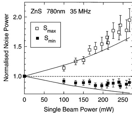
FIG. 4. Power dependence of the maxima ( $\square$ ) and minima ( $\blacksquare$ ) of the normalized phase dependent noise at 35 MHz. The solid lines show the results of Eq. (2) discussed in the text.
