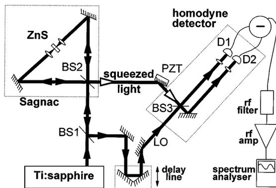
FIG. 2. Schematic diagram of the apparatus used to generate the squeezed light. BS1 is a 15% beam splitter; BS2, BS3 are 50% beam splitters. The piezoelectric transducer (PZT) is swept at 10 Hz and shifts the phase of the local oscillator (LO) relative to the squeezed light by several wavelengths. D1 and D2 are a matched pair of silicon photodiodes.
