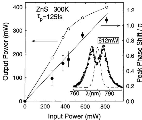
FIG. 1. Output power (○) and peak nonlinear phase shift (●) versus average input power at 780 nm. The solid straight line corresponds to  $|n_2| = 1 \times 10^{-14} \text{ cm}^2 \text{ W}^{-1}$ . The inset shows the output spectrum and fitted self-phase modulation curve (solid curve) at a power of 812 mW compared to the input spectrum (broken curve).
