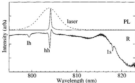
Fig. 3. Reflection (R) and luminescence (PL) of the 5 QW sample (see text) at  $T = 4$  K
