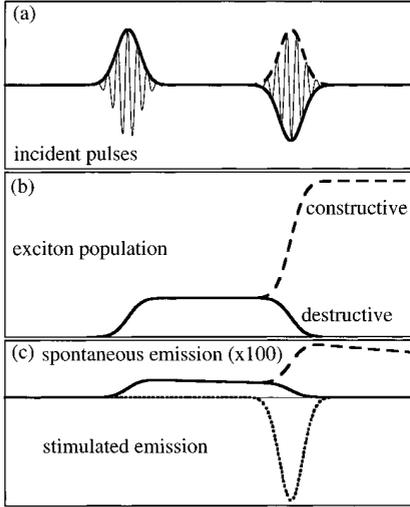
Fig. 1. Coherent control experiment. a) Incident pair of pulses are constructively- (dashed) or destructively-phased (solid). b) QW exciton density after excitation. c) Spontaneous and stimulated emission from the QW in the reflected direction as predicted by the semiconductor Bloch equations in the two scenarios
