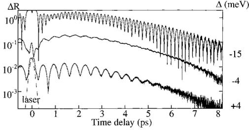
Fig. 4. Phase-dependence of the time-integrated reflection of the double pulse as a function of interpulse delay. The amplitude of the 2.67 fs period oscillations has been extracted and shown as a function of the detuning of the laser from the heavy-hole exciton ( $\Delta$ ). The upper two curves are shifted for clarity. Also shown (dashed) is the amplitude of the direct interference of the laser pulses
