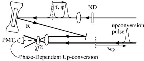
Fig. 6. Experimental scheme for up-conversion of the reflected light from the sample
