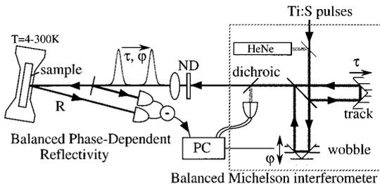
Fig. 2. Experimental scheme: pulses from an externally-recompressed mode-locked Ti:S laser are used to produce pulse pairs with variable but tracked temporal separation ( $\pm 10$  as)
