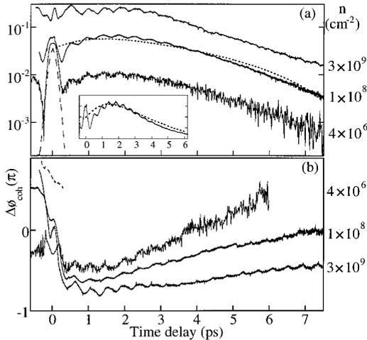
Fig. 5. a) Phase-dependent reflection of the double pulse at different incident intensities showing the rise and decay of the exciton coherence. The inset is for medium densities, plotted on a linear scale. The dotted curve is a fit from polaritonic interference in this sample using a purely radiative homogeneous linewidth, and an inhomogeneous linewidth of 0.2 meV. b) The extracted phase of the coherent reflectivity at different densities
