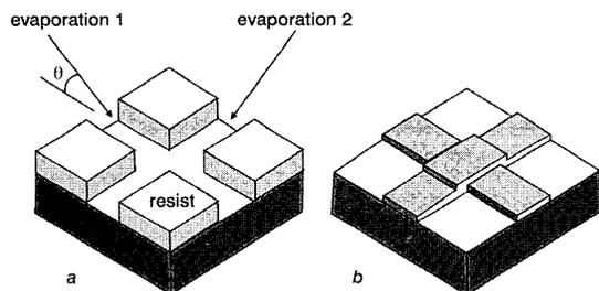
**Fig. 3** Schematic diagram of the single resist layer process
