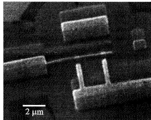
**Fig. 2** SEM image of a SQUID fabricated using the suspended shadow-mask method. The two evaporations (offset by  $1 \mu\text{m}$ ) can clearly be seen
