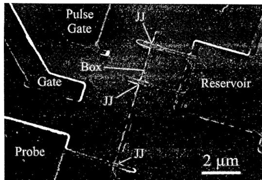
**Fig. 5** SEM image of a charge-coherent qubit fabricated using the orthogonal evaporation method, showing the Josephson junctions (JJ), the gates and the quasi-particle reservoir
