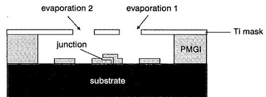
**Fig. 1** Schematic diagram of the cross-section through a shadow evaporation mask showing how by performing two successive evaporations at different angles a junction can be created
