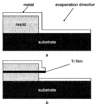
**Fig. 6** Schematic diagram of the resist cross-sections used in the lift-off process
