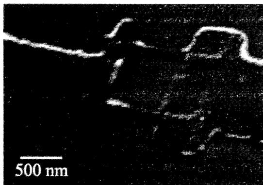
**Fig. 4** SEM image of a SQUID fabricated using the orthogonal evaporation method showing the two distinct levels of metallisation
