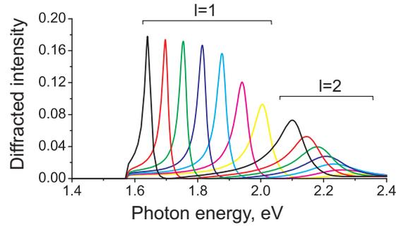
Fig. 5. Calculated intensity of the first-order diffracted beam with in-plane wavevector  $\mathbf{q}_{-1,-1}$  versus photon energy  $\hbar\omega$  for a surface of nanoporous gold formed by a hexagonal arrangement of spherical voids of different diameter  $d$ : from 380 to 500 nm (from right to left, in steps of 20 nm). The angle of incidence is  $50^\circ$ . The lattice constant ( $|\mathbf{a}| = 515$  nm) is kept unchanged in these calculations.
