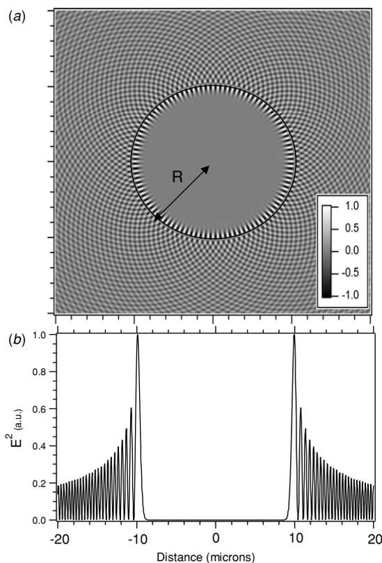
**Figure 3.** (a) A two-dimensional section of the optical field profile derived from a Mie scattering model of the  $l = 100$  TE WGM (arbitrary scale). The radius of the sphere is marked on for clarity. (b) Optical intensity along a radial direction, showing the evanescent mode leakage beyond the dielectric/air interface.
