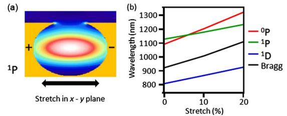
FIG. 3. (Color online) (a) Calculated field distribution of the  ${}^1P$  cavity mode in a 900 nm diameter nanovoid, which has been stretched by 20% in the  $x$ - $y$  plane.  $+/-$  indicate positions of charge nodes on the cavity walls. (b) Calculated energy of localized modes upon cavity stretching.
