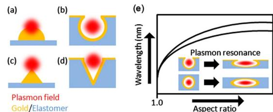
FIG. 1. (Color online) Hybrid metal-elastomer nanostructures and schematic resonant plasmon fields for (a) hemispheres, (b) voids, (c) tips, and (d) pyramidal pits. (e) Characteristic theoretical resonant plasmon wavelength dependence on structure aspect ratio (lines). As structures stretch, the broken symmetry results in plasmon splittings. Inset: schematic cavity with plasmon field distribution (shaded) when viewed from (top) side-on and (bottom) top-down.
