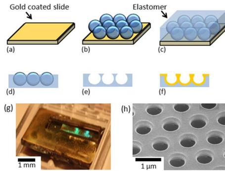
FIG. 2. (Color online) (a)–(f) Metal-elastomer nanovoid fabrication procedure. (g) Image of a typical sample, opalescent strip is nanostructured with nanovoid cavities. (h) SEM images of  $\bar{t}=0.8$  structure.
