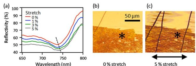
FIG. 4. (Color online) (a) Reflectivity of the metal-elastomer nanovoid structure with applied strain (dashed line indicates the wavelength of peak plasmon absorption). (b) and (c) Microscope images at  $10\times$  of (bottom) nanovoids and (top) flat metal on elastomer at strains corresponding to (b) 0% and (c) 5% stretching. Spectra in (a) taken at  $*$ .
